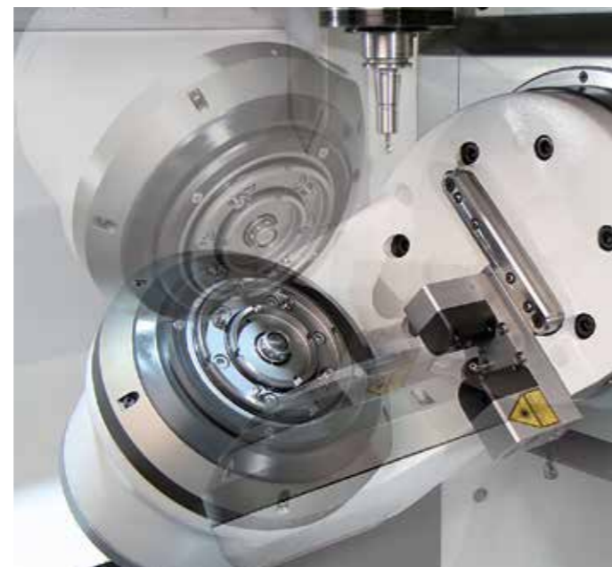
/// Pallet with coined cams
