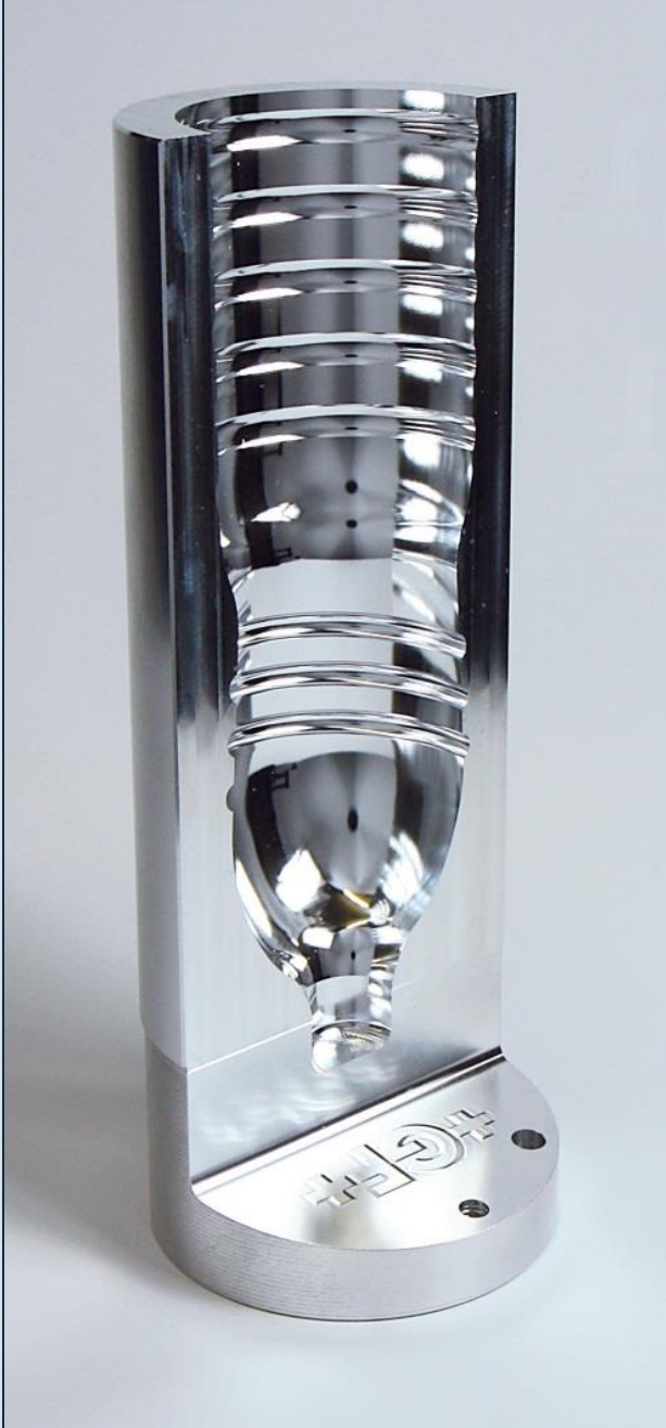
Bottle Mold, Headlight Mold, Golf Ball Mold machined without any secondary post processes
